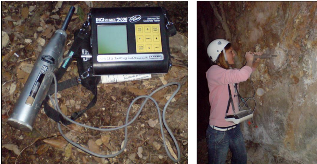
Figure 21 : Schmidt Hammer « Original Schmidt, N Type » (left), operator using the Schmidt Hammer on the cliff face (right)
