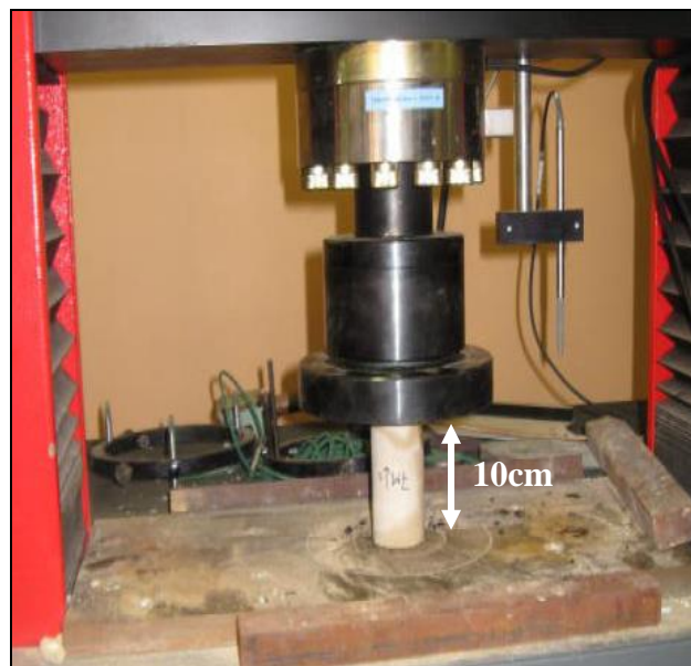
Figure 32 : UCS test with IGM Press with a 300kN captor. Specimen h=10\text{cm} , \varnothing=5\text{cm}
